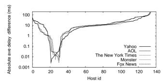
Figure 10: Latency gains for all measured PL nodes.
