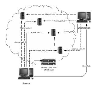
Figure 11: Illustration of the measurement methodology.
